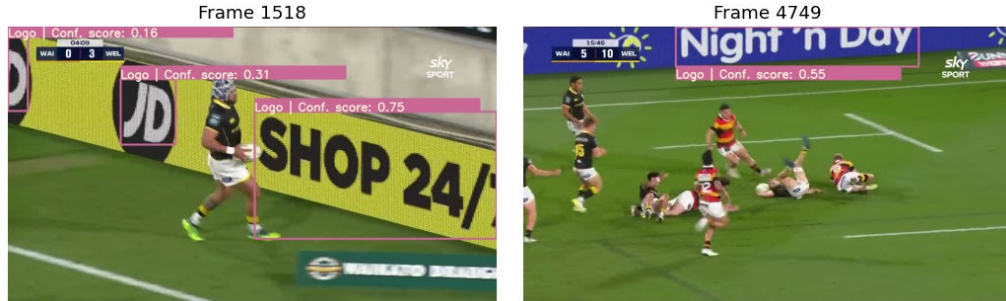
Figure 3: Example of detected logo with their confidence score. Only those with confidence scores higher than the threshold will be transferred to the tracking stage.
